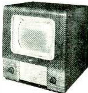
(Above) Philips projection television receiver, Model 600A, giving a picture 13\frac{3}{4} \times 10\frac{1}{4} in.
